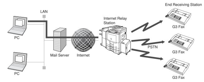
The Internet Relay Station (your machine) must be properly setup with all the required parameters.
